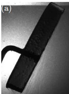
Dissolution of a submerged block of caramel. The flow is induced by solutal convection (Cohen et al. 2016)
